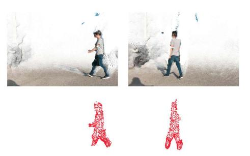
**Figure 6.** Moving obstacle detection (wandering pedestrian). In this test, both the person and the AGV were moving. (**Top**): original point clouds; (**Bottom**): detected clusters.
