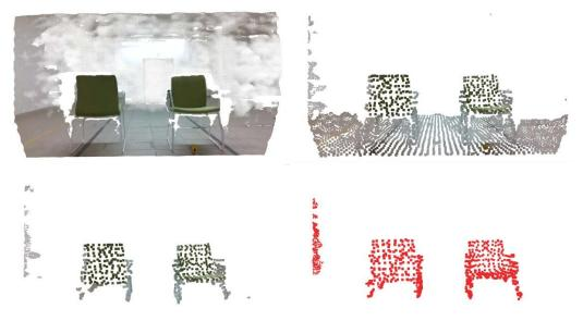
**Figure 3.** Indoor results for the four stages of processing. From top-left to bottom-right: original point cloud, down-sampled and range-limited point cloud, point cloud after ground plane removal and point cloud with detected clusters (two chairs).
