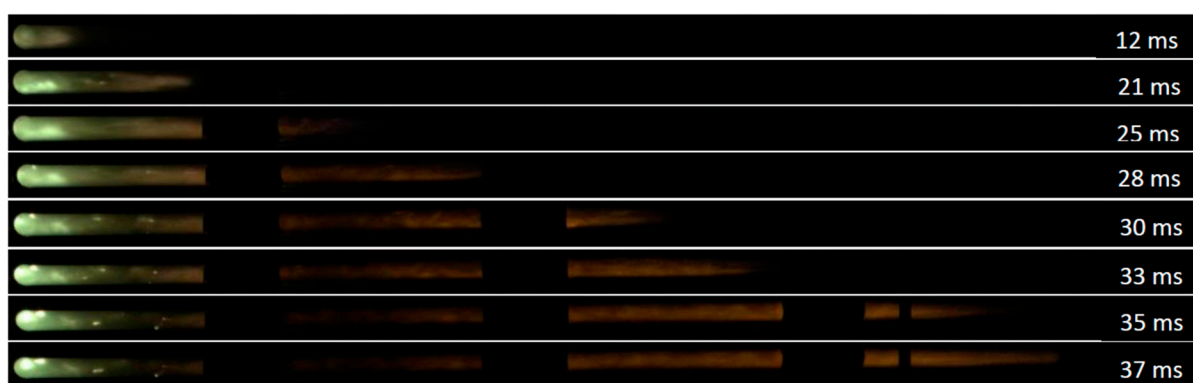
Figure 12. 10% methane–air flame propagation in the tube with a 70% circular opening obstacle positioned 1.2 m from the ignition source.
