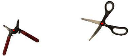
Fig. 6. Revolute axis estimation of pliers (left) and scissors (right) in 2D found by our method. The red dot indicates the estimated axis of rotation.
