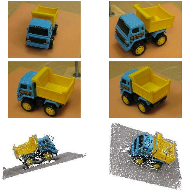
Fig. 4. Four images (out of 112 captured) of a toy truck. The last row shows the 3D reconstruction (two different views) obtained by the structure-from-motion procedure. An occlusion-aware model is produced in which points on the back side, as well as the front, are recovered.
