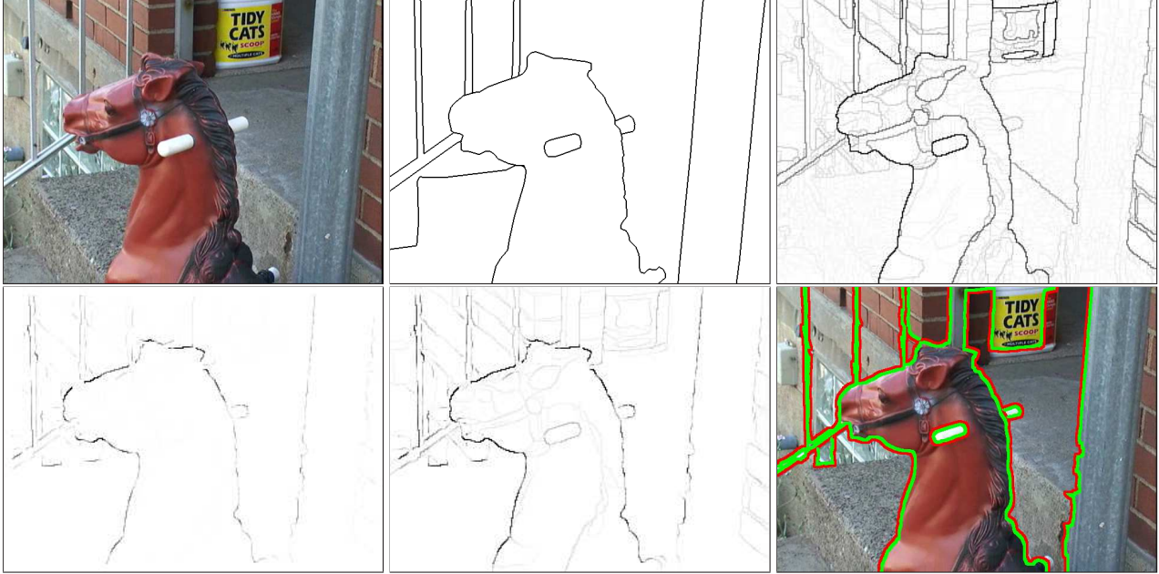
Figure 2. Overview. Top: Keyframe from the rocking horse sequence of [24], along with ground truth and the output of the static boundary detector of [2]. Bottom Left: Our motion feature \delta , computed on boundaries. Bottom Center: Resulting boundaries combining \delta and static cues. Bottom Right: Figure/ground classification results on detected regions, figure in green.
