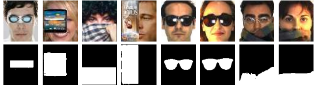
Figure 6. Occlusion detection results of our FCN-8s segmentation network on the occluded Facesub and AR test images.
