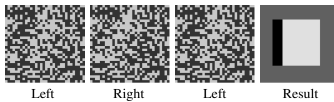
Fig. 7. Random-dot stereogram. Shown as result is the disparity map for the left image. Note the occluded region (black) at the left of the rectangle.
