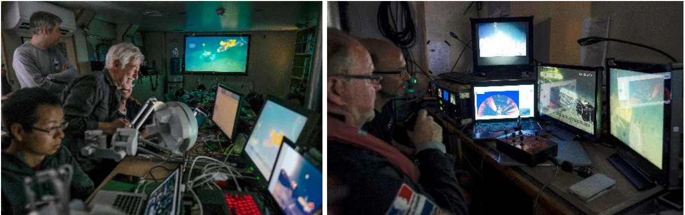
Fig. 13. The control room on-board André Malraux for this mission included the haptic-visual interface for Ocean One as well as views from other vehicles accompanying the robot during the mission.
