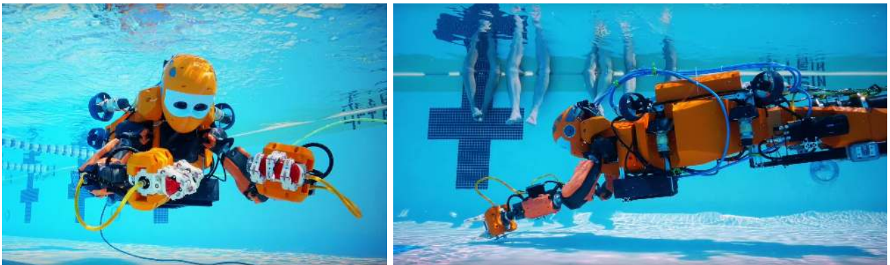
Fig. 10. Ocean One swimming at the Aquatic Center at Stanford University. This pool environment was used to adjust buoyancy and perform various validation tasks.
