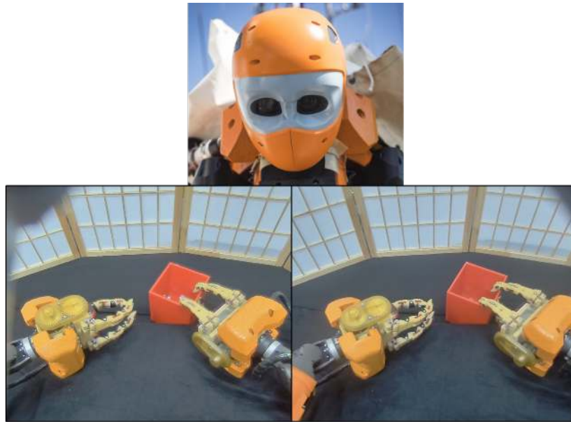
Fig. 9. Binocular-stereo cameras positioned at the robot's eyes stream to a passive 3D screen that immerses the operator in the task scene. A body-mounted camera (not shown) provides a wider alternative view.
