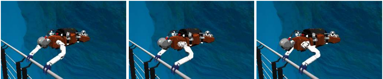
Fig. 4. Ocean One delivering a plastic crate. The body employs 8 thrusters, 4 on each side. Floatation foams create a neutrally buoyant platform. Spring-loaded oil-filled pressure compensators ensure that if a small leak occurs, the robot compartments do not take on water.
