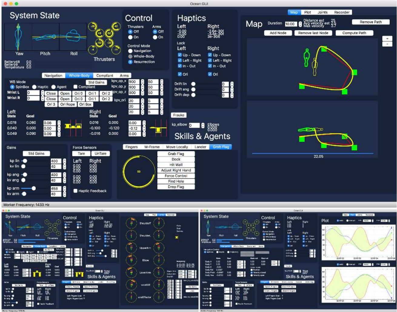
Fig. 11. The graphical User Command Center allows the user to monitor system state, select control modalities and plan manipulation tasks. Top: System state display - roll-pitch-yaw, depth, estimated linear planar position, thruster forces. Radio buttons for control mode selection. Push buttons and spin boxes for control parameter tuning. Interactive map that allows the operator to set trajectory control points (green squares), trajectory generation (yellow path), robot-state (green outline), robot-goal (yellow outline). Bottom-Left: Circular dial widgets displaying joint-space control state (red), goal (yellow), torque (green). Bottom-Right: Functionality for live plotting and recording for offline analysis.
