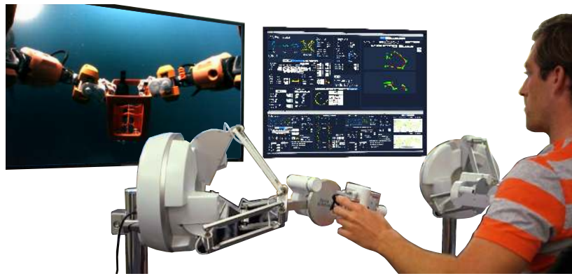
Fig. 3. A human operator guiding the robot in an underwater bimanual task through the haptic-visual interface consisting of two Sigma.7 haptic devices [8], a stereoscopic 3D display, foot pedals and the graphical user command center.
