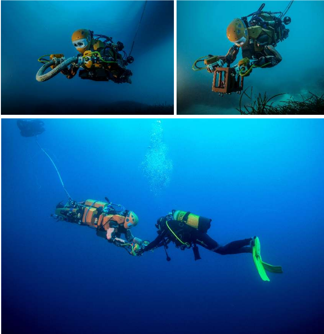
Fig. 14. Ocean One diving in the Mediterranean at 15 m: grasping objects (top) and interacting with the diver in a compliant and safe manner (bottom).
