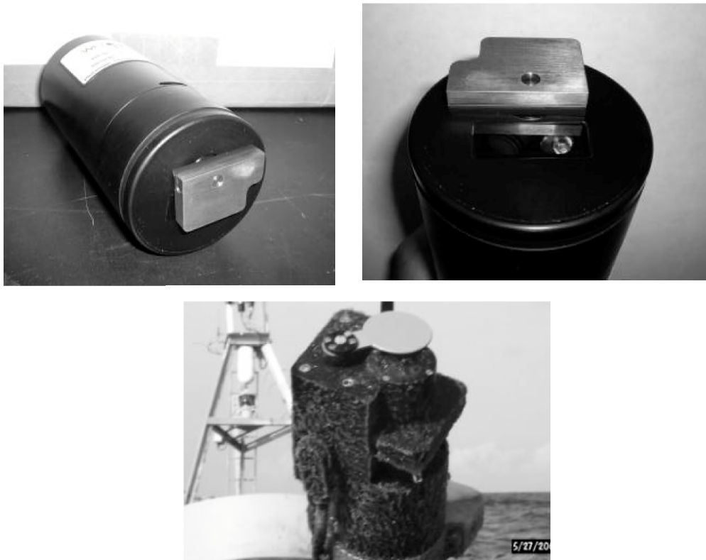
Fig. 3.13. Examples of optical instruments equipped with copper shutter mechanisms to protect the optical windows from bio-fouling. A new instrument is shown in the upper panels with its shutter closed (left) and open (right). The lower panel shows biofouling organisms covering a different instrument, except for its copper shutter, upon recovery from a moored deployment.
