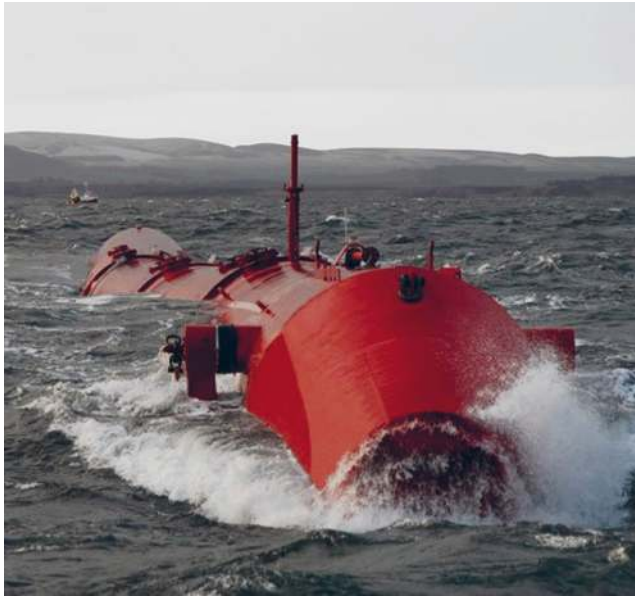
Figure 1.4: An oscillating body device, the Pelamis wave energy converter.
