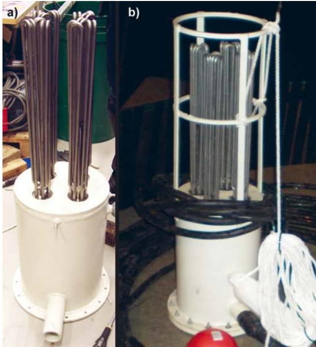
Figure 4.8: (a) A dump load during construction. (b) The dump load of L3 being prepared for deployment.
