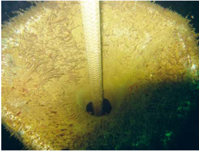
Figure 4.5: Vectran-cored buoy line with a Dyneema cover running through the stainless steel funnel in the top of WEC L1. The funnel supports the line in the horizontal plane to protect the piston rod sealing in the top lid of the capsule from this stress.
