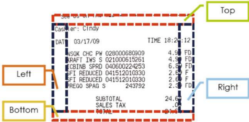
Fig. 2. Four 10-pixel wide margins
