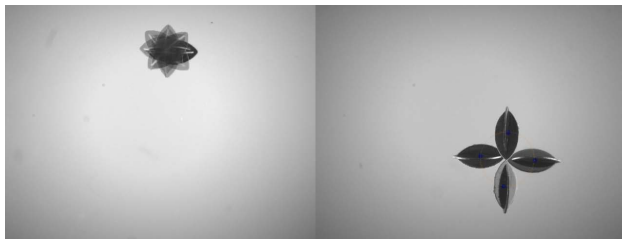
Fig. 2. Demonstration of rotation control. Both time-lapse image sequences show a single 2-mm-long microrobot in the z = 0 plane (viewed from above). The left image sequence demonstrates rotation of the microrobot in place at an arbitrary location in space by relying on pure open-loop control. The right image sequence demonstrates rotation of the microrobot about a remote center at an arbitrary location using closed-loop control.
