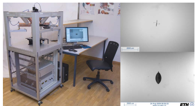
Fig. 1. The OctoMag prototype contains eight 210-mm-long by 62-mm-diameter electromagnets. The gap between two opposing electromagnets on the lower set is 130 mm. The insets are the top and side-camera views, and show a 2-mm-long microrobot of the type described in [5].
