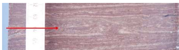
Fig. 6. Figure showing probable gas escape during and after sedimentation of laminae at depths of 630 to 645 mm.
