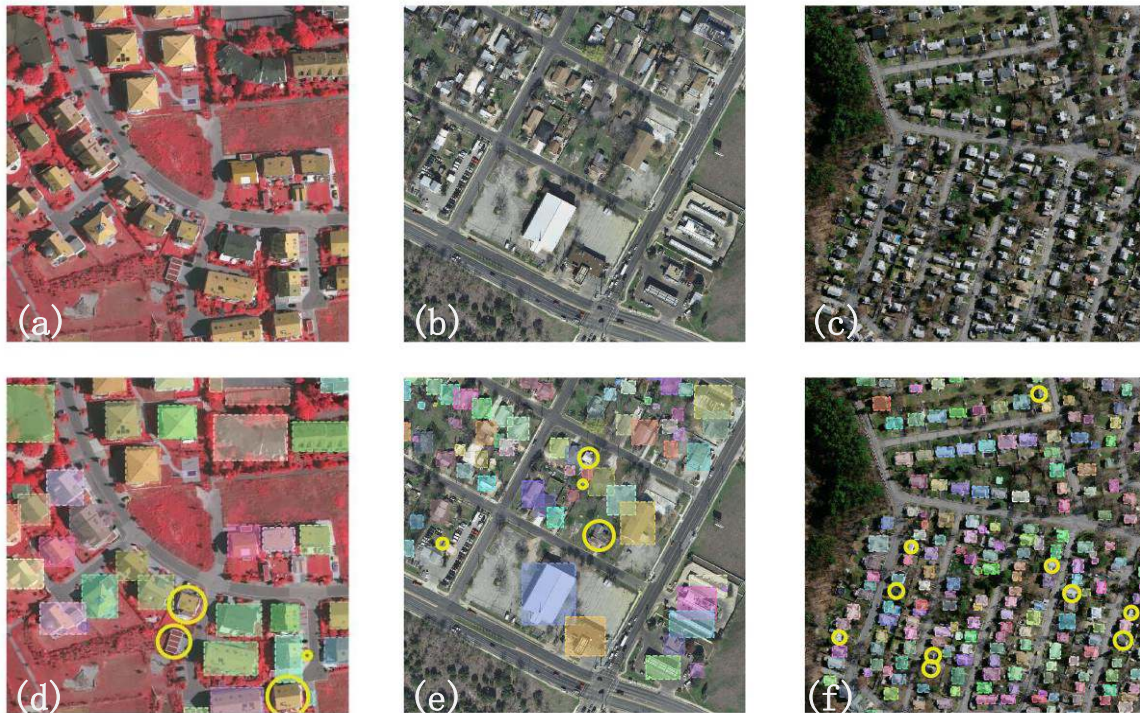
Fig. 9. Results of object detection using the Mask R-CNN. The first row shows three images from the three datasets, respectively, i.e., (a) image of ISPRS, (b) image of INRIA, and (c) image of Massachusetts building datasets. The images coupled with localized buildings are shown in the second row, i.e., (d) object detection results of the image in (a), (e) object detection results of the image in (b), and (f) object detection results of the image in (c).
