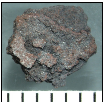
Figure 6.10. The flake depicted here is typical of deteriorated iron and is found throughout the wreck site and across the region (photo R. Horlings, 2008).
