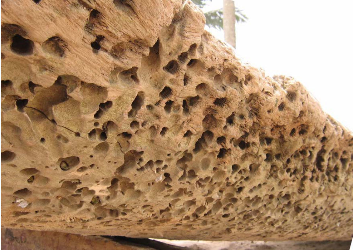
Figure 6.7. The holes in this dug-out canoe base which washed on shore near Elmina were likely drilled by molluscs such as the Teredo : there is clearly a weakening in the structure of the wood as a result of all of the borings. Because wood-boring organisms thrive in warm waters (Pournou et al 2001), the risk of severe damage by these organisms increased with the amount of time a wooden sailing vessel remained in the tropics. Wood in similar condition was collected in sediment cores (see Core GW#2 in Appendix I) from the shipwreck site, indicating that it was exposed for a period before collapsing and being covered up (photo R. Horlings, 2007).
