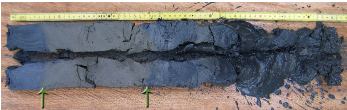
Figure 4.5. Splitting the core reveals the complex stratigraphy of a site: the sediment color, texture and contents change with depth, indicating different environmental and cultural processes and events; sediment changes are highlighted by green arrows. The left side is the top of the core, the right the bottom (photo R. Horlings, 2007).
