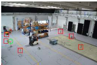
Fig. 38: Measurement setup. The industrial environment consists of metal shelves and industrial vehicles. The Receiver/Anchor tags are highlighted with red boxes, the transmitter/mobile node is highlighted with a green circle.
