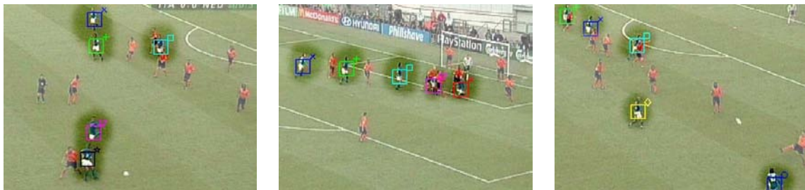
Fig. 4. Tracking in action on the soccer sequence. Only the blue team is tracked, other areas are in lower contrast. Videos are available at [8]. (Image courtesy of Rádio e televisão Portugal)
