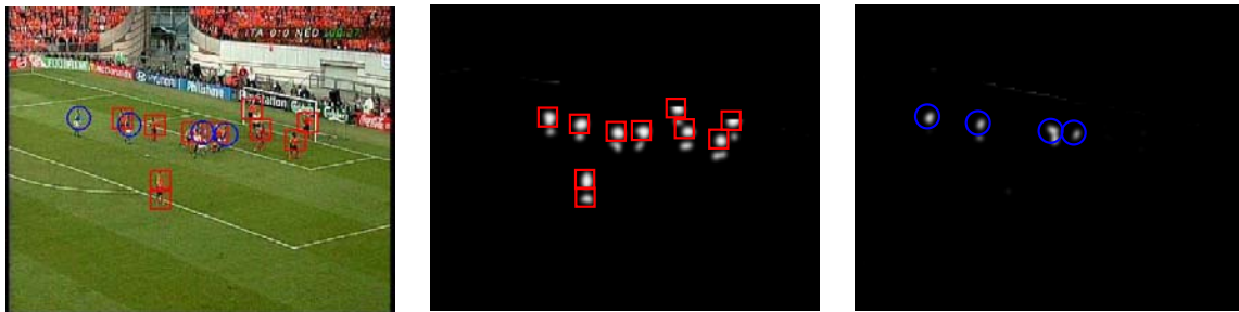
Fig. 3. Example of Player Detection using colour segmentation and MeanShift to find the blobs centres.
