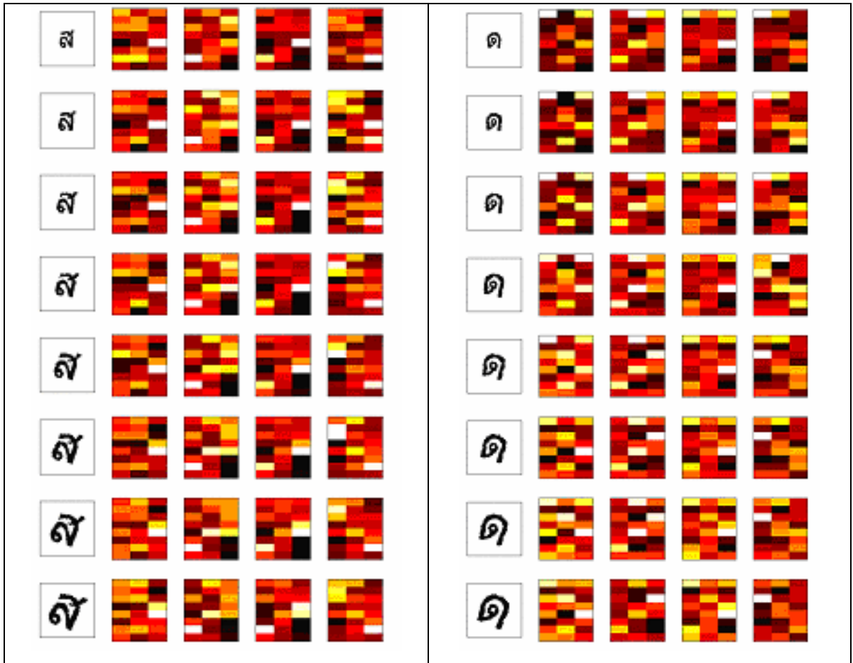
Figure 4.25 Variation of printed characters [ஸ] and [ட] with their corresponding edge direction features.
