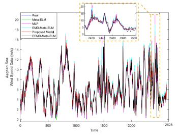
Fig. 10. Forecasting test results of Aegean Sea.
