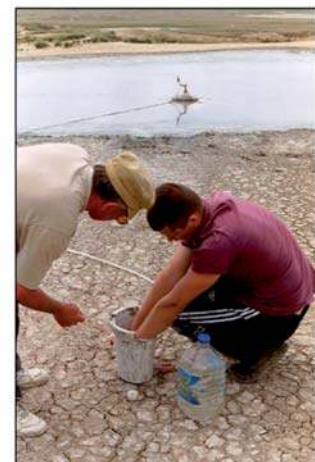
Figure 11 Launch of the "Chapka Monomaha" and sampling of gas samples 10 m away from the bubbling point on Pavlov.
