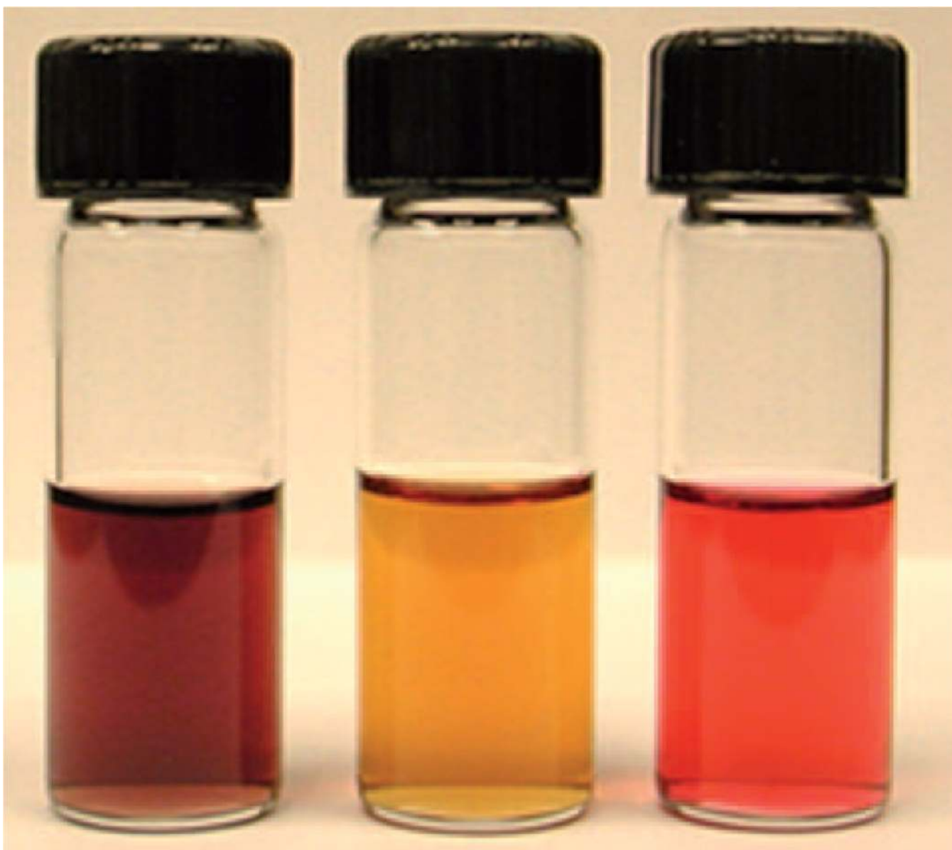
Figure 1. Photograph showing the color changes seen upon the addition of uranyl acetate to solutions of isoamethyrin. Left: Acid salt of isoamethyrin; Middle: After addition of 10 equivalents of \text{Et}_3\text{N} . Right: \text{UO}_2^{2+} complex. Solutions of uranyl acetate and isoamethyrin were made up using a 3:4 (v/v) mixture of methanol and dichloromethane. This figure, which originally appeared in reference [24], is reproduced with permission.
