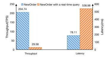
Fig. 1. This figure reveals the impact of a hybrid workload – performing a real-time query in-between an online transaction on the performance of TiDB – a state-of-the-art HTAP system against that of only an online transaction. The significant performance gap justifies why we should consider real-time queries in benchmarking HTAP systems. The other two critical factors that the HTAP benchmarks must consider are semantically consistent schema and domain-specific workloads.
