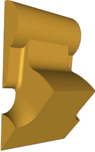
Fig. 5. A computer model for one eighth of the vacuum part of a DDS cell.
