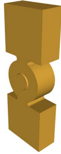
Fig. 6. A computer model for a cavity coupled with two identical rectangular waveguides.
