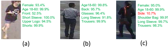
Figure 7. Likelihoods on ground-truth attributes predicted by OSNet. Correct/incorrect classifications based on threshold 50% are shown in green/red.
