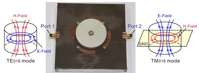
Fig. 1. Prototype of the proposed dual polarized omnidirectional DRA with schematic field distributions for the two orthogonal modes excited.
