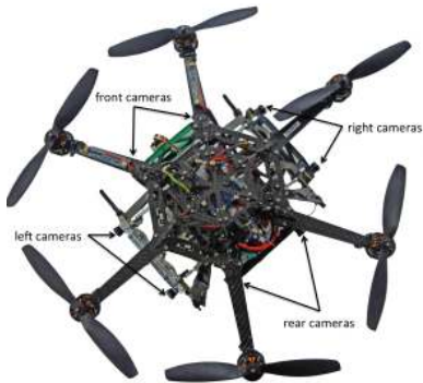
Fig. 3: AscTec Firefly platform with mounted eight camera setup. The four stereo camera heads are targeted towards different directions to cover the surroundings of the MAV.
