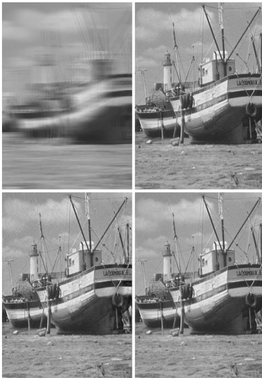
Fig. 3 In this experiment, we assume that the scene s moves at velocity v = 1 pixel per second. The additive (readout) noise is Gaussian with a standard deviation equal to 10. We also assume that the scene emits 625 photons per seconds (for other values see Table 1) On the top left panel: the observed image using the Agrawal and Raskar code [5,6]. On the top right panel: the observed image for snapshot an exposure time of 1 second, i.e., the blur support is 1 pixel. On the bottom left panel: the reconstructed image for the Agrawal and Raskar code [5,6]. On the bottom right panel: the reconstructed image for the snapshot (blur support of 1 pixel). This means that for the Agrawal and Raskar code the blur has a support of 52 pixels. In other words, this code permits to increase the exposure time by a factor 52 compared to the snapshot. The RMSE using the Agrawal and Raskar code is equal to 9.84. The RMSE of the snapshot is equal to 5.96. We refer to Table 1 for different values of mean photon count and additive (readout) noise variance. This simulation is based on a variant of [29]
