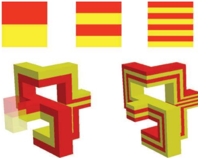
FIG. 1. (Color online) Top: baker's transformation of the unit square after two iterations. Bottom: sketch of mixing action of the present flow after two elements.
