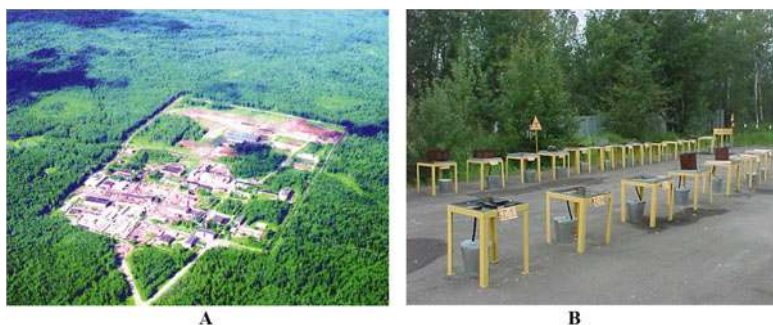
Fig. 3. (A) An aerial view of testing site; (B) Nuclear waste glass samples BS8, BS, 9, BS10 on open testing area
