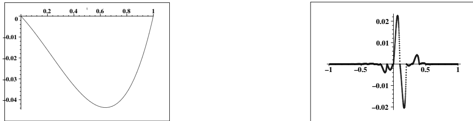
Figure 3: Plot of the basic function \omega_j^{<-3>}(x) (left), and the error of approximation of the Runge function with the polynomial splines, h = 0.1 , x \in [-1, 1] (right)
