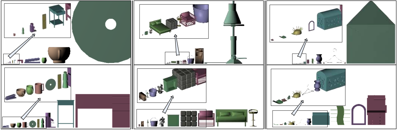
Figure 8: Three sets of models selected through sorting by bounding box diagonal, binning into 10 bins and randomly sampling from the central 10% of each bin. Top: models in original scales. Bottom: Corrected scales using our Combo algorithm (unsized models in gray).
