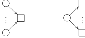
Figure 3.5: Free-choice nets: the two subnets from which any free-choice system can be built.
