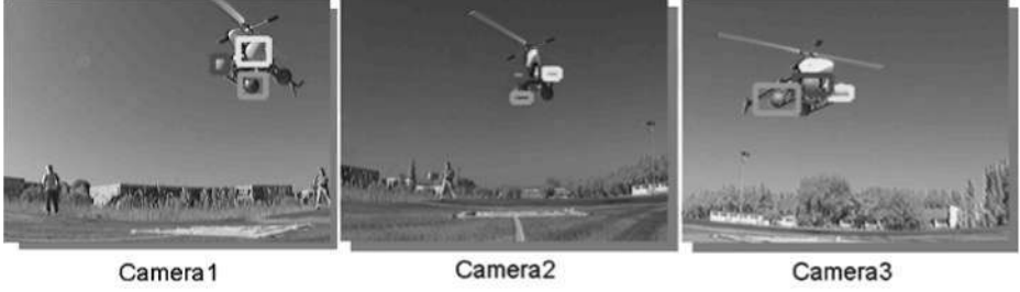
Fig. 3 Feature extraction in the trinocular system. Color-based features have been considered as key-points to detect the UAV
