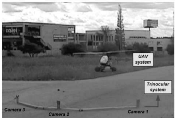
Fig. 10 Trinocular system and Helicopter testbed (Colibri III) during a vision-based landing task
