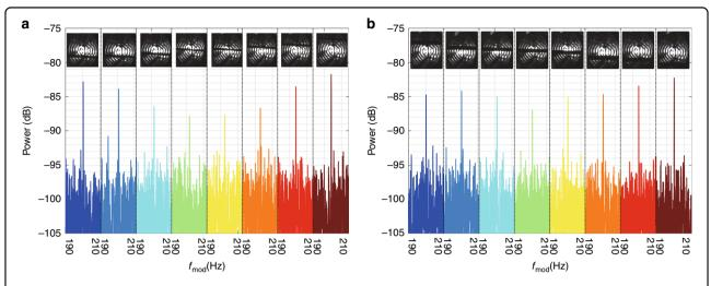
Fig. 5 The rotation speed measurement with obstacles. a The obstacles are cylindrical copper wire with a diameter of 1.18 mm and b 2 mm. They are 0.801 m away from the chip surface, and the rotation speed is 100 r/s. The power spectral line in each cell is measured under the light spot condition above the cell
