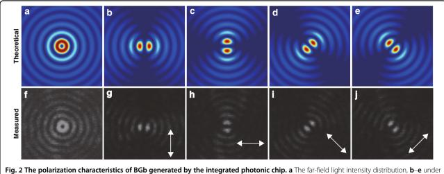
Fig. 2 The polarization characteristics of BGb generated by the integrated photonic chip. a The far-field light intensity distribution, b–e under different polarization states, theoretically. f Measured intensity distribution at a distance of 2.2 m from the chip surface, g–j after a polarizer in the directions indicated by the arrows
