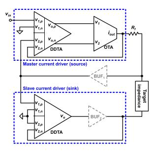
Fig. 22. A closed-loop current driver employing simple source and sink current drivers [8], [115]–[117]. The BUF<sub>1</sub> is used in [115], [116] and the BUF<sub>2</sub> is used in [117]
