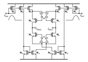
Fig. 19. An output stage of open-loop current driver with the regulated cascode output stage [111].
