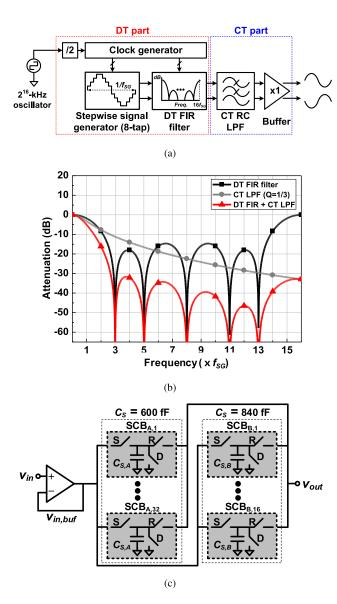
Fig. 17. A SSG based on DT FIR filter [45]: (a) a block diagram of the overall architecture, (b) frequency responses of the DT and CT filters, and (c) a block diagram of the DT FIR filter.
