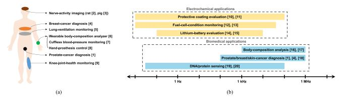
Fig. 1. (a) Biomedical applications of impedance measurement and (b) applications of electrical impedance spectroscopy and their required frequency ranges.
