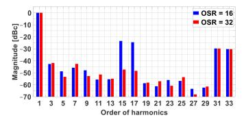
Fig. 5. Simulated harmonic magnitudes of a sinusoid generated by a 6-bit DAC with an OSR of 16 and 32.
