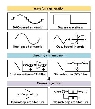
Fig. 3. Three main stages of on-chip SSGs and representative techniques for each stage.
