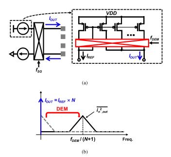
Fig. 8. (a) A square waveform generator based on a single-bit current DAC whose current source employs a dynamic element matching (DEM) technique. (b) Noise characteristics of the square waveform generator with DEM.
