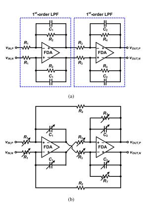
Fig. 13. Example active RC filters: (a) a 2nd-order active RC LPF for an on-chip SSG [47] and (b) a 2nd-order Tomas biquad RC LPF [103].
