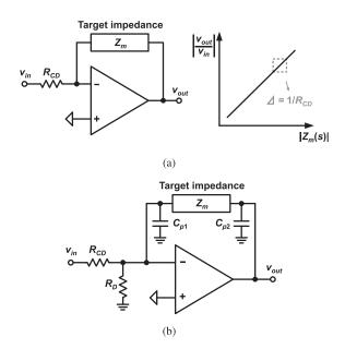
Fig. 20. (a) A closed-loop current driver based on the auto-balancing bridge and the gain ( $\frac{V_{\rm out}}{V_{\rm in}}$ ) over the target impedance [89] and (b) a loop-stability compensation scheme for this structure [89].
