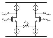
Fig. 18. An open-loop current driver using the source degeneration [5], [28], [84], [85].
