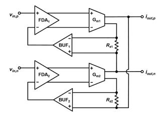
Fig. 21. A closed-loop current driver with a linear feedback [113].
