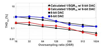
Fig. 6.  $\,$  THD  $_{\!13}$  versus OSR for 8- and 6-bit DAC cases in comparison with the calculated 1/SQR  $_{\!13}.$
