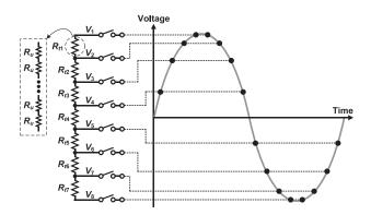
Fig. 7. Operation principle of a sinusoidally tapped resistor DAC for sinusoidal waveform generation. The resistor chain with only eight taps is demonstrated for simplicity. In [51], [52], 33 taps with 1000 unit resistors were used.
