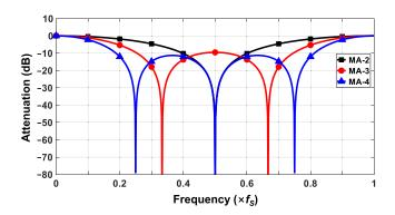
Fig. 16. Frequency responses of moving average (MA)-2, MA-3, and MA-4 filters
