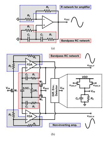
Fig. 9. Two sinusoidal oscillators based on Wien-bridge architecture: (a) a single-ended design [82], [83] and (b) a fully differential design [5], [28].
