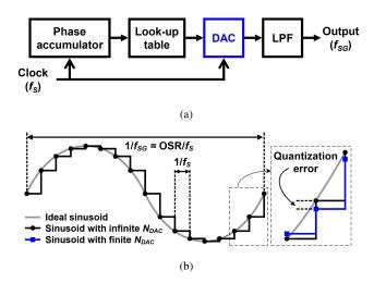
Fig. 4. (a) Block diagram of direct digital synthesizer for generating DAC-based sinusoid [46] and (b) an example DAC-based sinusoid when OSR = 16.  $f_{SG}$  is the frequency of the generated sinusoidal waveform, and  $f_S$  is the sampling frequency. OSR =  $f_S/f_{SG}$ .
