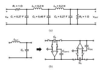
Fig. 15. (a) The 5th-order Chebyshev type-I LPF using LC ladders with 1-Hz  $f_{C,LPF}$  and 0.5-dB pass-band ripple [24] and (b) implementation method of a LC pair with SC circuits [24].
