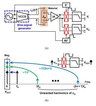
Fig. 2. (a) Block diagram of general on-chip EIS systems. (b) Error caused by the signal harmonic folding at the frequency mixing stage in the demodulator.
