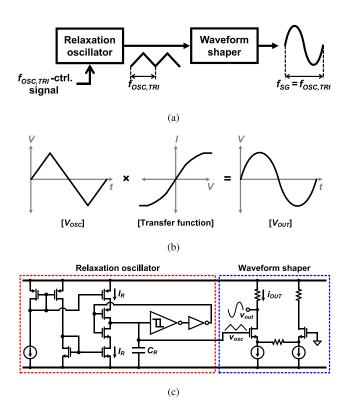
Fig. 11. (a) The block diagram of SSGs based on oscillator-based triangular waveform [90]–[92], (b) an operation principle of the waveform shaper [92], [93], and (c) a schematic of the SSG based on oscillator-based triangular waveform for EIS [92].
