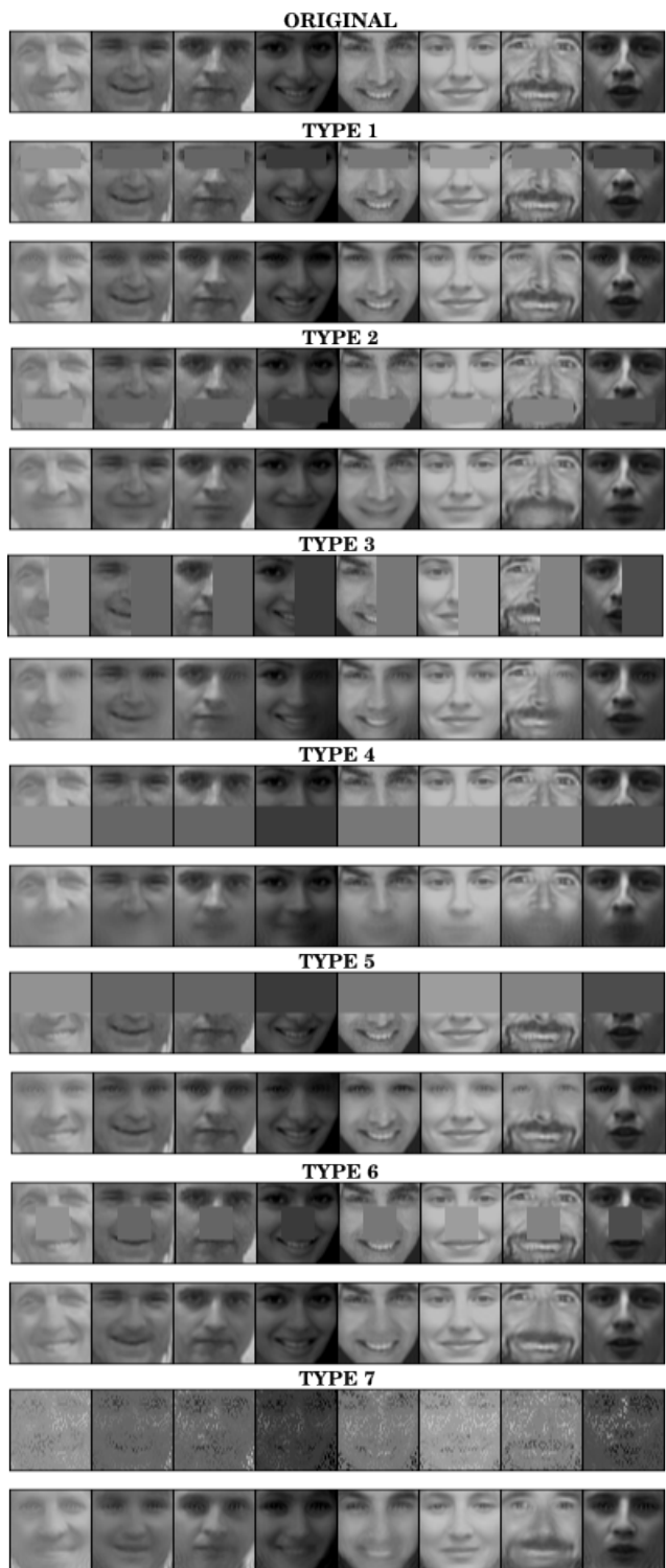
Figure 5. Example of conditional generation performed by a four-layer deep model trained on faces. Each column is a different example (not used in the unsupervised training phase). The topmost row shows some example images from the TFD dataset. The other rows show the same images occluded by a synthetic mask (on the top) and their restoration performed by the deep generative model (on the bottom). We consider seven types of occlusion. Afterwards, we use the restored image to predict the facial expression of test identities.
