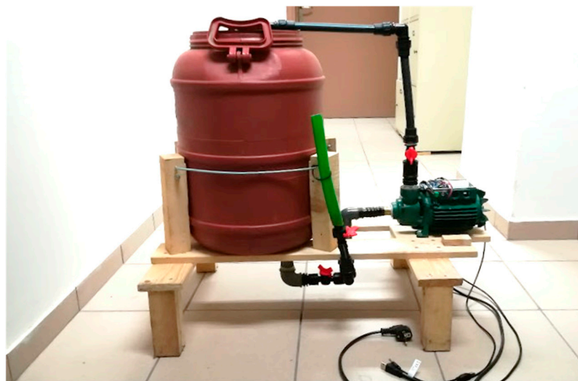
Figure 3. The implementation details for the proposed system, including a centrifugal water pump and three intervening plastic valves in the piping.
