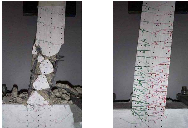
Fig. 11 Damage behavior of (a) R/C and (b) R/ECC without stirrups, shown at 10% drift. Even at this high drift level, no spalling of the ECC was observed. In contrast, the R/C column lost the concrete cover after bond splitting and spalling occurred.
