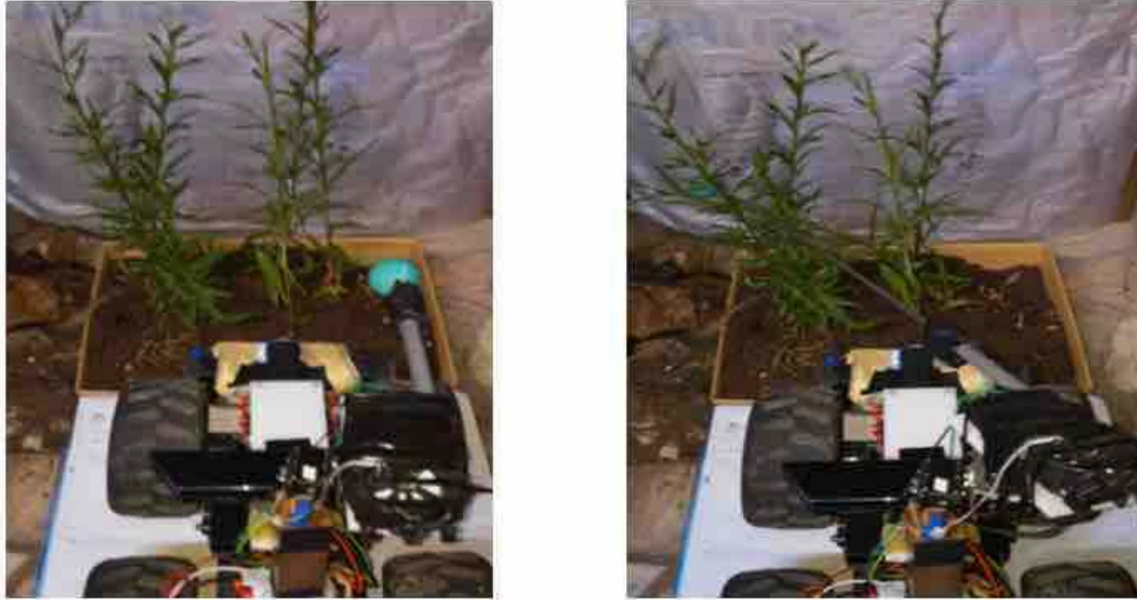
Figure 8: Typical haptic interaction execution. The antenna stretches to the distance of the furthest interaction point then follows the plan. Note that this behaviour results in a scanning pattern that bends traversable obstacles.
