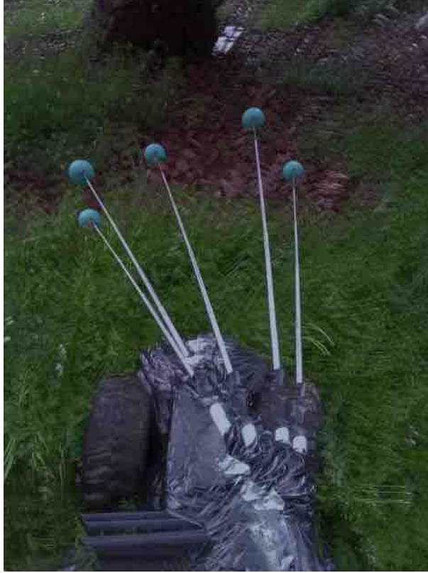
Figure 5: Time lapse image of the babbling behaviour used to learn the rigid transformation between the range sensor and the antenna frames of reference.
