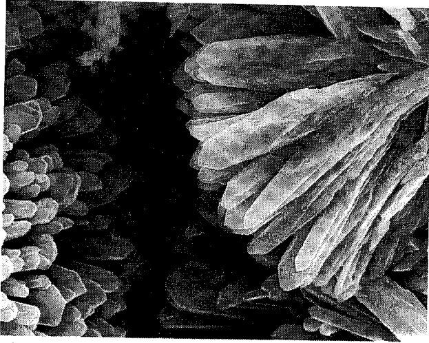
Fig. 2. GaN crystals grown in synthesis process at T = 550^{\circ}\text{C} , p = 5 kbar, \text{Ga}:\text{K}:\text{NH}_3 = 1 : 2 : 20 .
