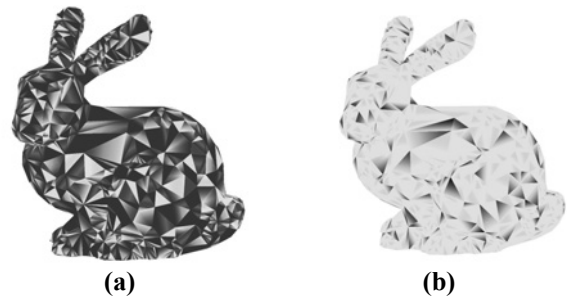
Figure 7: Visualization of rendering performance of a locality-preserving rendering sequence. Light vertices incur no cache misses. Dark vertices incur many cache misses. (a) Using random ordering, ACMR = 2.65. (b) Using MLA-induced rendering sequence, ACMR = 0.71.
