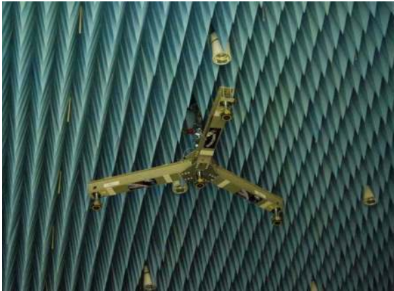
Fig. 12. Test jig with four probes in the ceiling of the Maxwell anechoic chamber at ESA-ESTEC.
