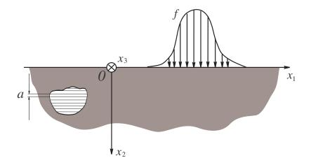
Figure 1: Antiplane shear of a nonlocally elastic half-space.
