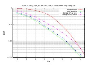
FIG. 3 – BLER for 2 users/interf cell : filtered demap-remap
