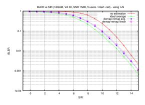
FIG. 4 – BLER for 5 users/interf cell : filtered demap-remap
