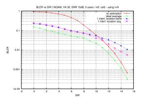
FIG. 2 - BLER for 5 users/interf cell : interferer location
