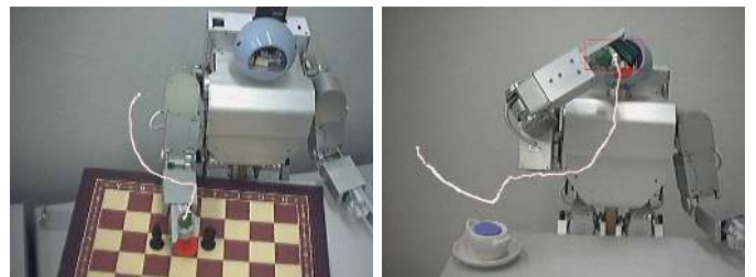
Fig. 10. Experimental results for the Chess Task and Sugar Task , when performed under different situations than the ones demonstrated (different final position on the chessboard and different head pan/tilt). The trajectory of the hand was tracked by the vision system, and superimposed to the image.
