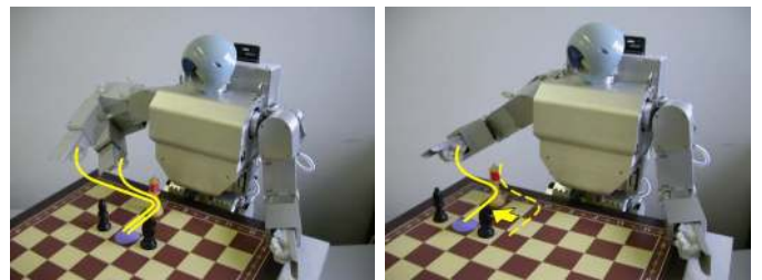
Fig. 2. Left : Illustration of the what-to-imitate issue. With two demonstrations of a Chess Task , we see that the constraints are varying along the motion. To approach the chess piece, a large set of paths are possible, depending on the initial position. Grabbing and pushing the piece requires higher constraints, i.e. the paths do not change much between two consecutive demonstrations. Right : Illustration of the how-to-imitate issue. To re-use the learned skill in different situation (here, different position of the chess piece), a cost function is used to select a controller that best fulfills the task constraints along the trajectories.
