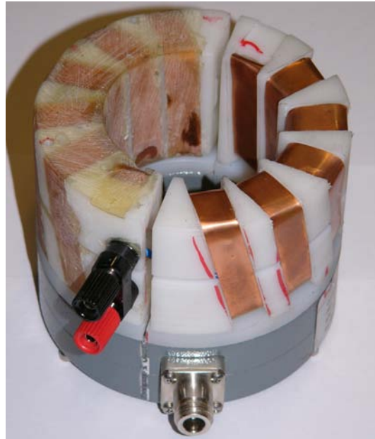
Figure 4.22 Photo of the designed injection coil, mounted to a commercially available measurement coil (Fischer CC F-70)
