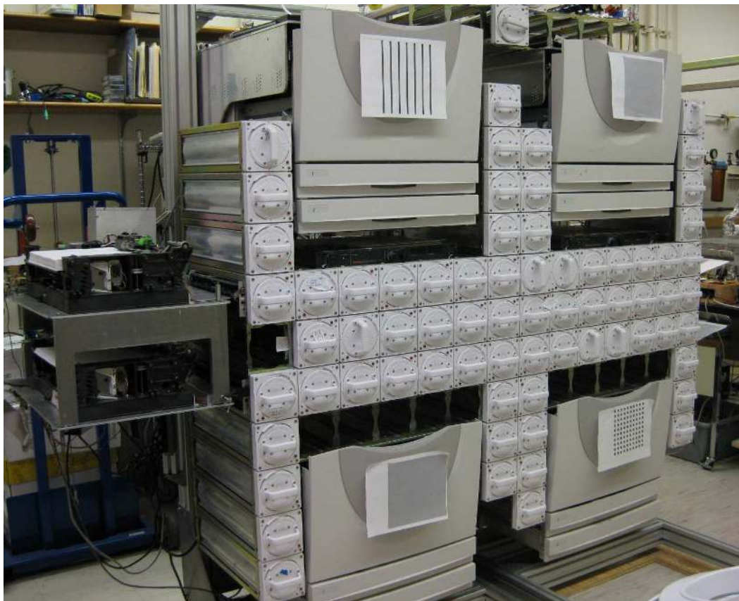
Figure 1: A prototype modular printer built at PARC. The system is composed of approximately 170 individually controlled modules, including four print engines.
