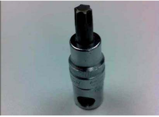
Fig. 16. Torx 45: a typical industrial end-effector tool.
