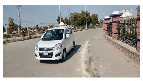
**Figure 2.** Instrumented test vehicle containing a roof-mounted antenna along with a PolaRx5s multi-frequency and multi-constellation GNSS receiver as used for field experimentation and data acquisition.
