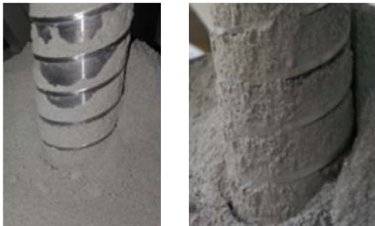
a Rotary speed: 200 r/min b Rotary speed: 85 r/min Figure 2 Simulant chips in the auger groove under different drilling parameters (Penetrating speed: 85 mm/min)
